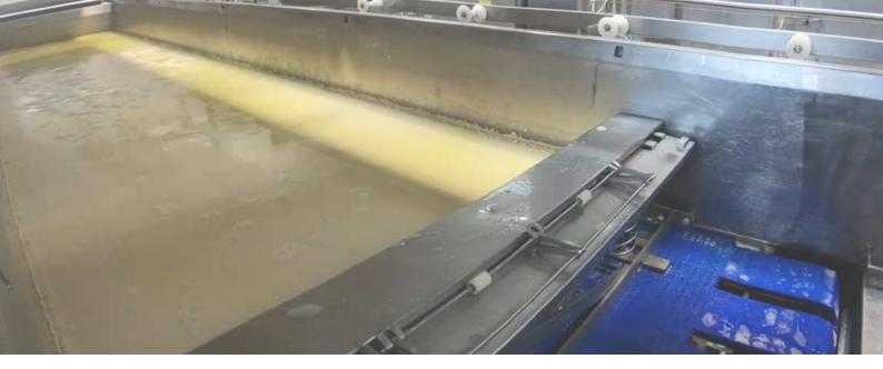
Premium quality cheeses depend on an even curd distribution, efficient drainage and prepressing and precise cutting according to a defined weight distribution. Even curd distribution and predictable weight, higher capacity with short changeovers and accurate traceability all contribute to higher revenues from a higher yield of premium quality cheeses.
